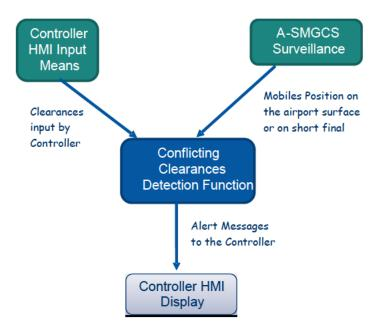
Figure 7 - Conflicting ATC clearances detection - Functional architecture
