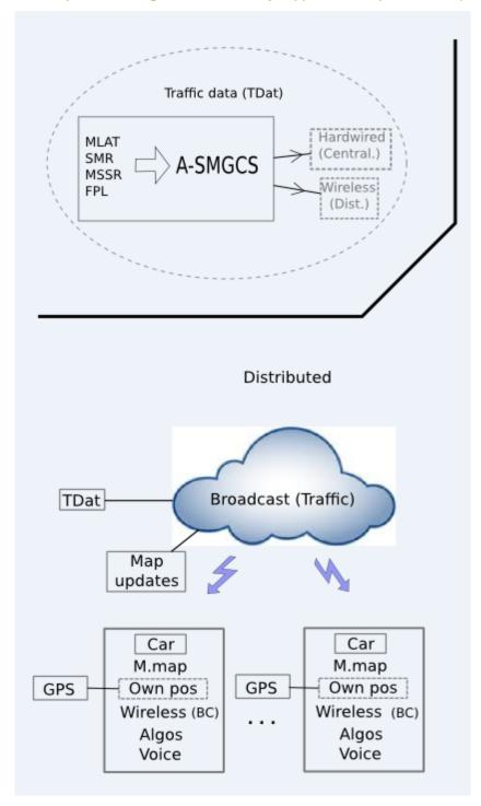
Figure 16 - Functional architecture for alerts directly generated on-board the vehicle
