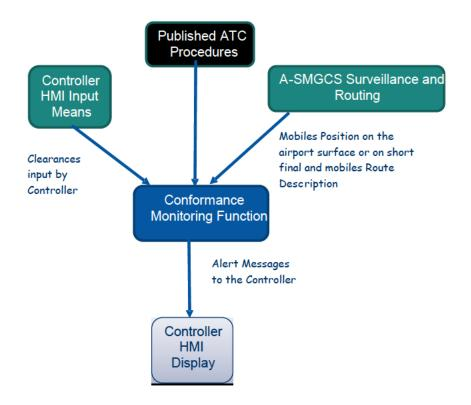
Figure 10 - Conformance monitoring alerts - Ground functional architecture
