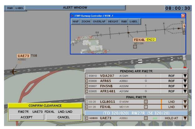
Figure 6 – Indication of a potential CATC in a warning window (example only, other implementations of this concept exist)
