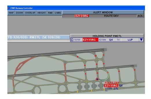
Figure 9 - Conformance monitoring alerts - Example of Route Deviation Alert 'ALARM'
